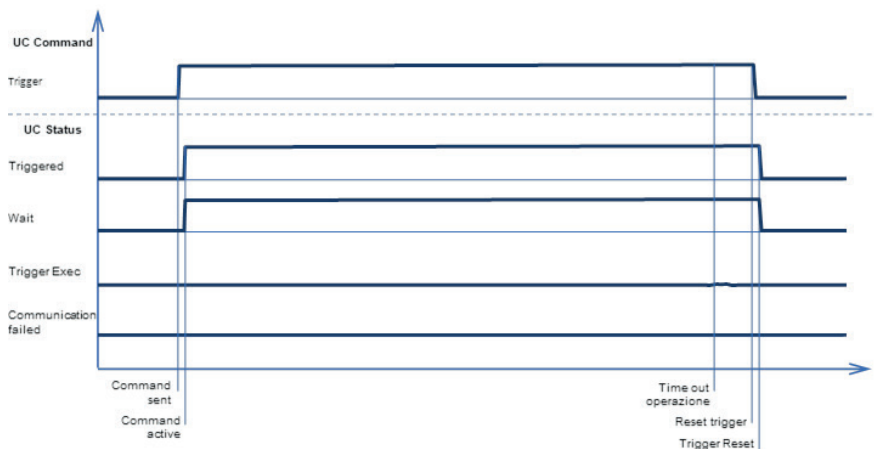
Fig. 10.5 – Timing flag in case of unreachable device
